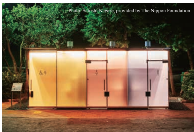
When the door is locked, the transparent walls become opaque, emanating warm, earthy natural tones.
