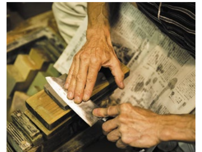
After sharpening the blades by machine, he refines their edges by hand.
