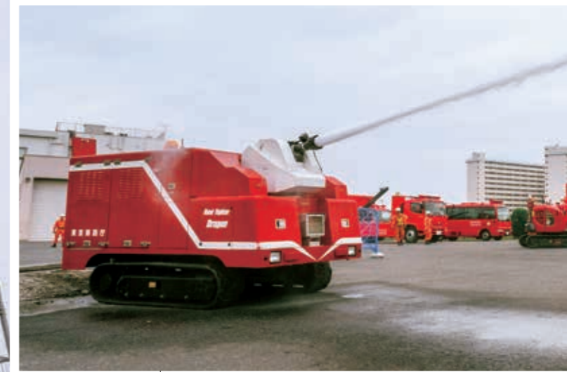
The remotely operated water discharging "Dragon" being deployed.
