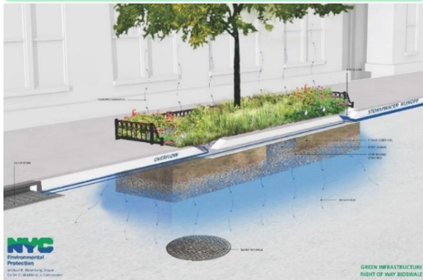
Storm water infiltration greenbelt (rain garden)
